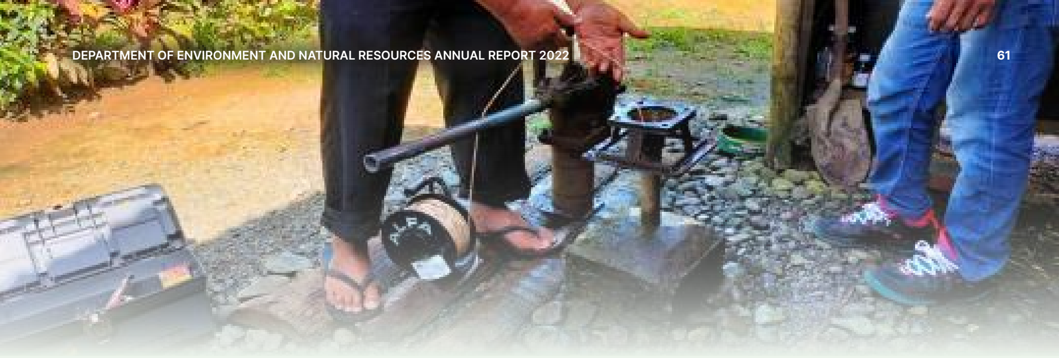
Measuring the water level of the private jetmatic pump, using ALFA WL 100 type-2B instrument located in Purok 5 of Barangay San Vicente, Madrid, Surigao del Sur.
