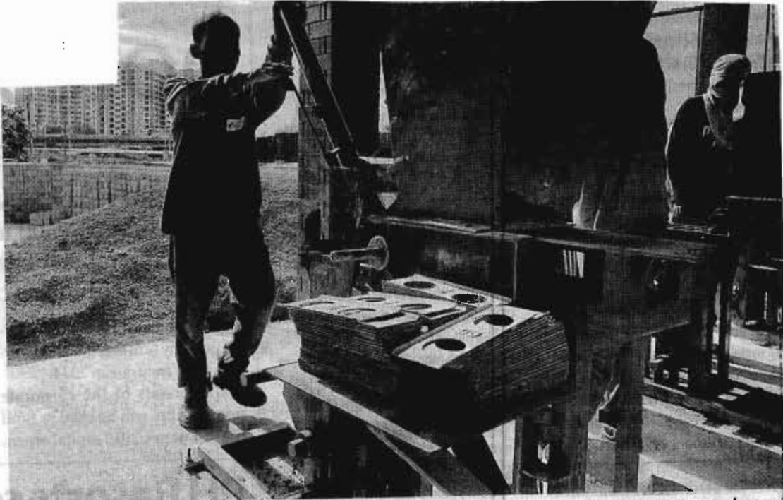
■ A man operates a brick-pressing machine that mixes shredded sachet laminates with wet cement to produce an ecobrick at a facility run by Green Antz Builders Inc. in Taguig City. XINHUA PHOTO
