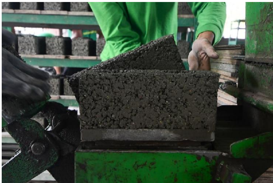
Workers produce bricks mixed with upcycled plastics at Green Antz' site in Plaridel, Bulacan. Mark Demayo, ABS-CBN News
