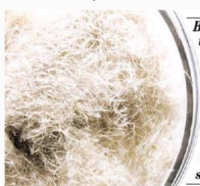
OPENED bamboo textile fibers.
