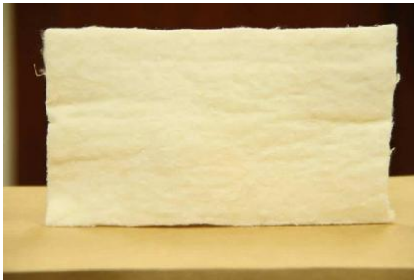
DOST-PNRI Radiation-Modified Abaca/Polyester Fabric (Photo from DOST-PNRI)
