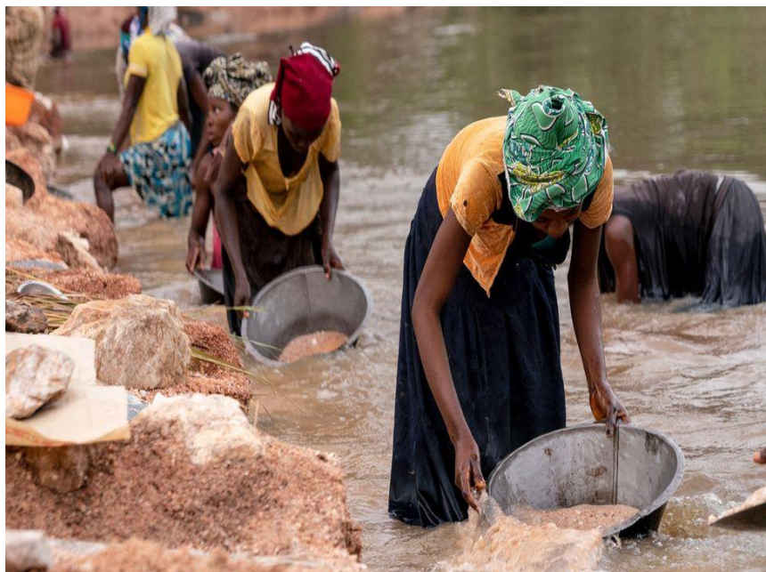
Artisanal miners collect gravel from the Lukushi river searching for cassiterite – the major ore of tin – in Manono, Democratic Republic of Congo (Credit: J.Kannah/Getty Images)
