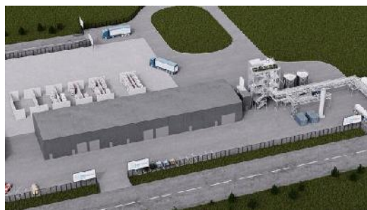
The plant that is being constructed at Teesside in the UK aims to process 80,000 tonnes of plastic waste every year (Credit: Mura)
