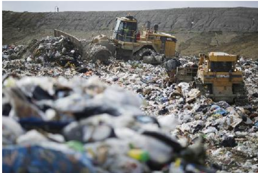
A Caterpillar Inc. 836G Landfill Compactor and D9T Dozer drive through garbage at the Waste Management Inc. Skyline Landfill in Ferris, Texas.
