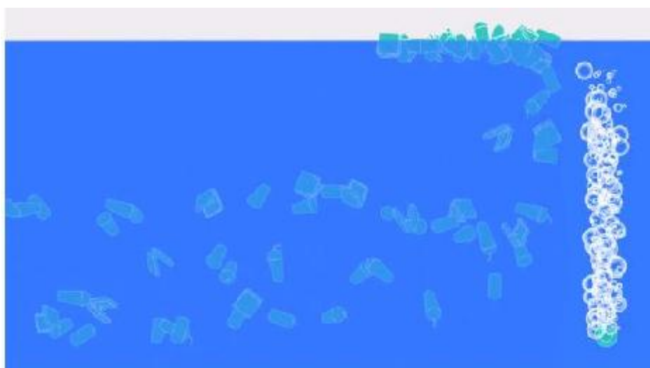
Trash is lifted to surface, and guided to a catchment system.
