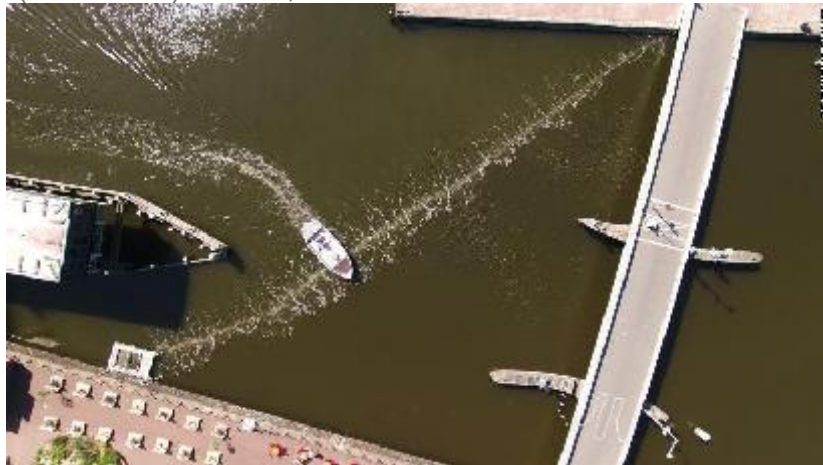
A boat passing through the "Bubble Barrier" in Amsterdam's Westerdok canal.
