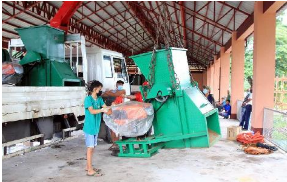
Pyrolysis gasification processing machines being set at the Dumaguete City's Central Materials Recovery Facility. (Contributed photo)
