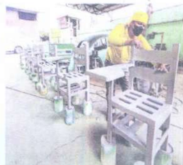
A worker from Envirotech is priming and sanding a school chair made from recycled plastic, getting it ready for painting.
