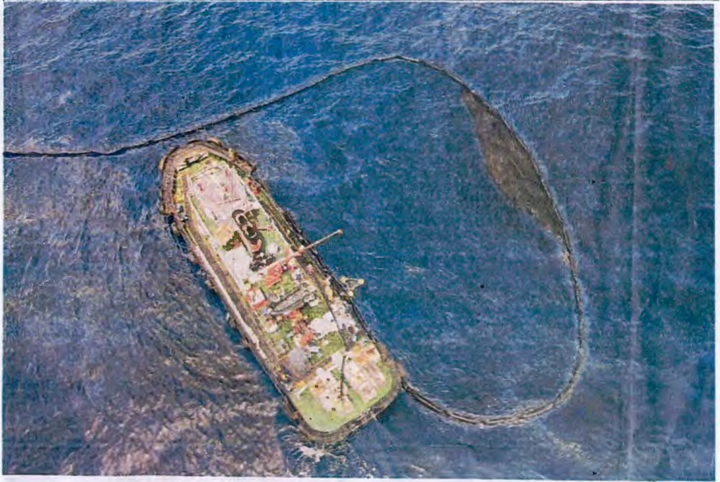
CONTAINMENT. The Philippine Coast Guard (PCG) reports two tugboats have deployed their oil spill boom and skimmer around the suspected area of the sunken tanker MT Princess Empress at six nautical miles northeast off the shoreline of Ballingawan Point and Buloc Bay in Oriental Mindoro.
