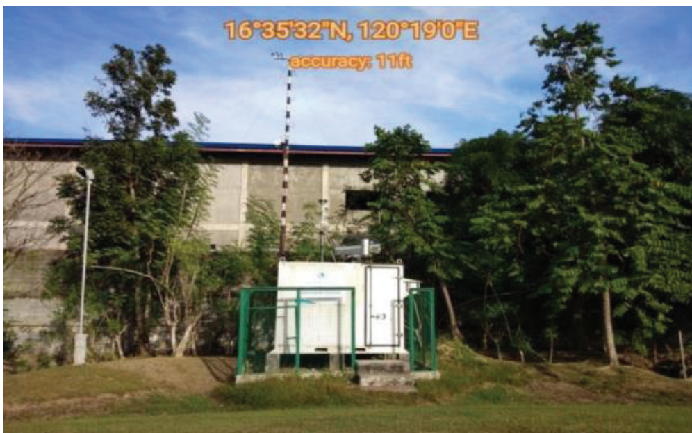
Figure 4.17 Ambient Air Quality Monitoring Station in San Fernando City, La Union (Region 1)
